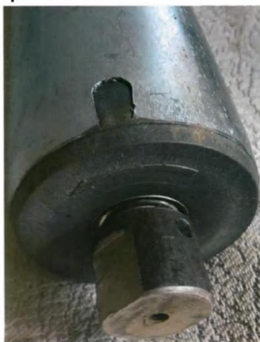
梳型托辊专用隔离套 (可根据尺寸切割) Special isolation sleeve for comb type idler ( can be cut according to size )
